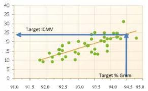
and IC-MV in order to correlate the production IC-MV values to the Department specified in-place air voids. A sample linear regression curve example is as follows.
